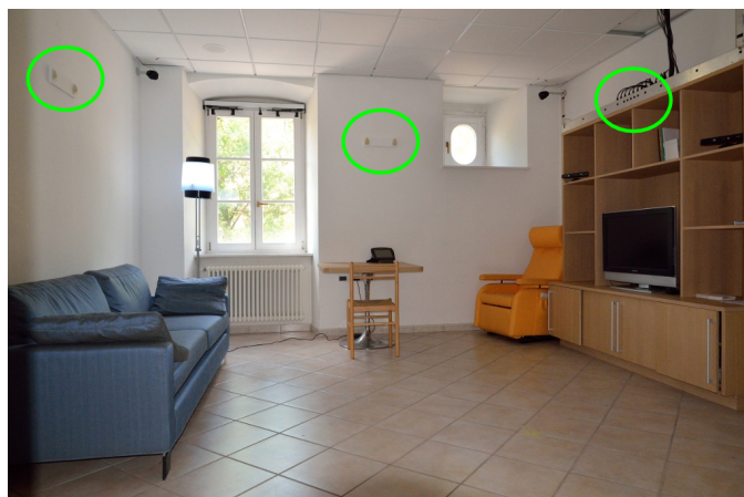
Figure 2.6: A photograph of the living room in the DIRHA smart-home. Some of the microphone arrays are marked by green circles.
